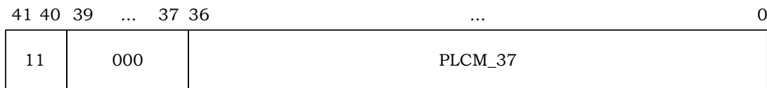
c) Public Long Code Mask for the Reverse Fundamental Channel with Radio Configurations 3, 4, 5, and 6, the Reverse Supplemental Channels, the Reverse Dedicated Control Channel, and the Reverse Common Control Channel in the Designated Access Mode
